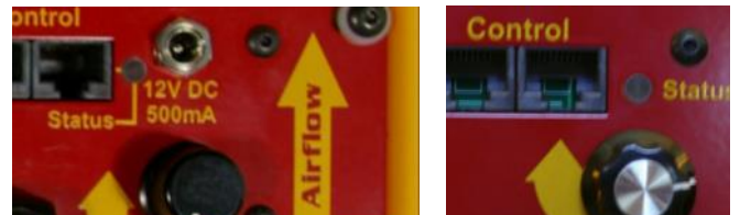
Figure 6: Speed Control Knobs on the Fan Tops of Door Fans. The Speed Control Knob of the 2350 Door Fan is displayed on the left, and of the 1000 Door Fan on the right.
