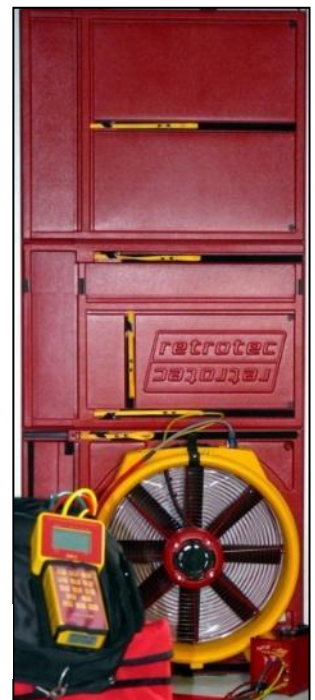
Figure 24: Modular door panel set installed.
