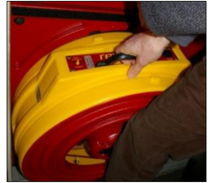
Figure 25: Installing a fan in a modular door panel set.
