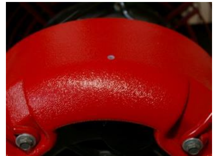
Figure 32: Pressure sensor on the fan motor casing.
