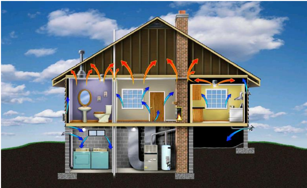
Figure 1: Stack pressure is caused by warm air rising and cool air falling.
