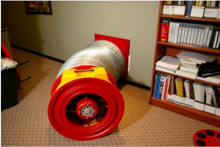
Figure 12 Flex attached to Blower Door
