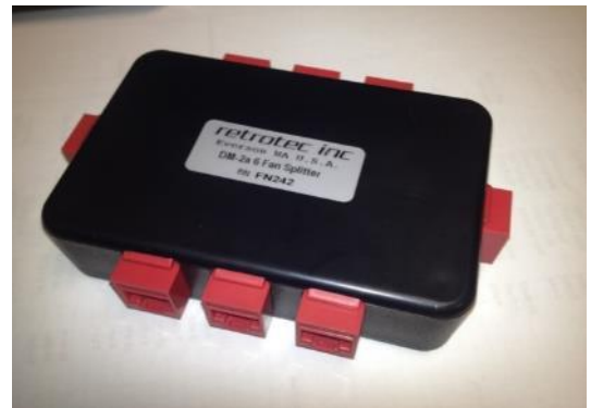
Figure 28: Current Speed Control Splitter (Part number FN280) works in all configurations.
