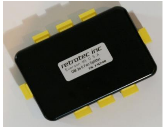
Figure 27: Do NOT use this older Speed Control Splitter with a computer connected to the gauges since the interconnectivity may cause damage to your computer. (Part number FN242) works in some configurations. See the Multi-Fan Manual for instructions.
