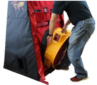
Figure 12: Installing a fan in the cloth door panel.
