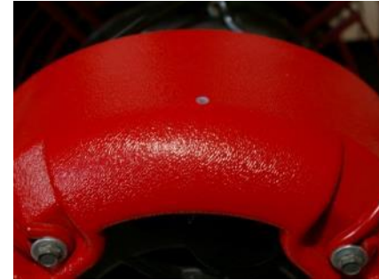
Figure 18: Pressure sensor on the fan motor casing.
