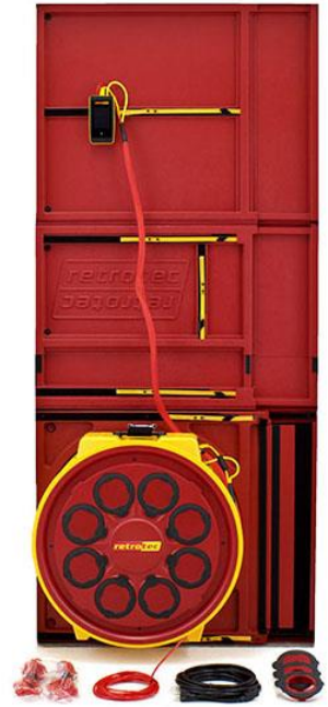
Figure 14: Modular door panel set installed.
