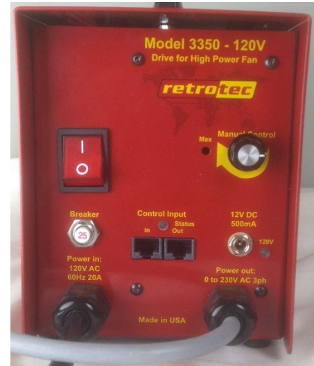
Figure 30: Cable ports on Model 3350 fan drives from 2012 and later.
